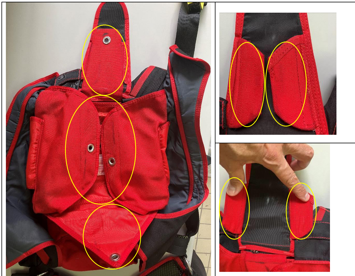
Figure 1 - Zone de chevauchement des rabats adhérentes / Adherence area of flaps overlapping
