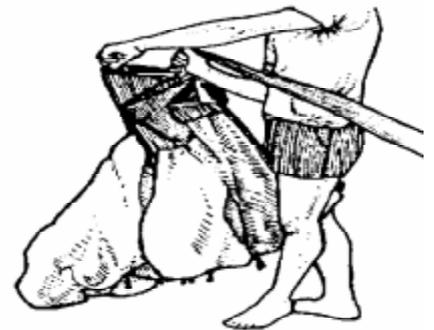
**14)** Find the group of A lines on one side of the canopy. With the canopy held in front of you as you have it now, the A lines are the front part of the line group that go through the front slider grommets, the ones that should be closest to you.
