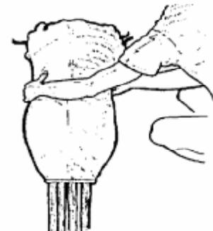
**31 & 32)** Move to the side of the canopy and put one hand right under the slider edge of the bundle. Place the other hand on top a little farther up and make a small S-fold as shown. Be sure the slider stays up against the stabilizers; don't let it move down the lines.
