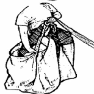
**20)** Now grasp the steering lines where they attach to the tail, pull the entire tail out and drop it straight down. "Quarter" the slider and leave it in its position.
