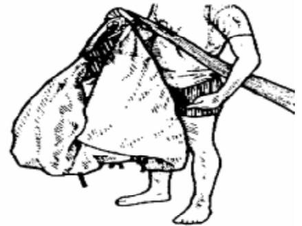
**13)** Clear the stabilizers. Since all lines are bunched up in the middle, pull each stabilizer panel out one by one into a loop until they form an irregular shape resembling the petals of a flower when viewed from the top. Be sure none of the lines are wrapped around a slider stop on a stabilizer.
