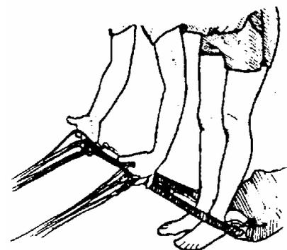
**2)** At this point you can determine if your canopy and lines are straight. If there are twists in the lines as shown, this means your rig "looped" through your risers at some point. To fix this, drop the lines, stretch the canopy and lines out again and straighten the entanglement out. Get help from a rigger if you have any questions. Do a line check again to make sure you have done it correctly.
