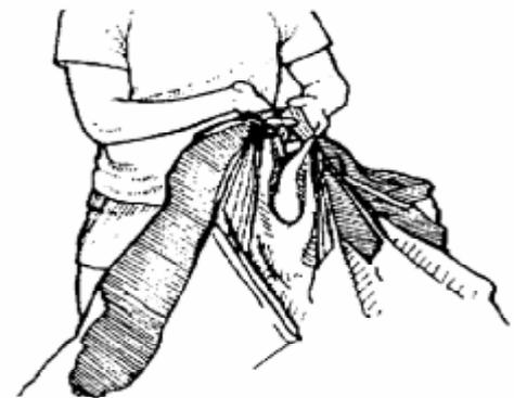
**6)** Now step to one side outside the lines and transfer the lines to one hand so that the left and right sides of the canopy hang at the same height. It is not necessary to keep the line groups separated by the fingers of your hand because you've already determined the lines and canopy are straight. Your canopy should look like the illustration. All lines should be kept taut and the nose should still be facing the rig. The slider should be against the slider stops on the stabilizers.
