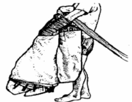
**16)** Now that you've pulled out the canopy between the A and B line groups, do the same thing between the B and C lines. Pull the fold of fabric between the two groups out to each side. When you look down in between the stabilizer folds after you've done your "flaking" the folds should look neat like this.
