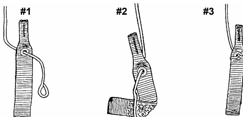
Route the steering line through the slider, then the toggle guide ring and then the toggle. **See drawing #1.** Thread the toggle through the loop in the steering line. **See drawing #2.** Pull loop up to the toggle grommet. Note that the loop of the steering line is going through and around the toggle. **See drawing #3.**
