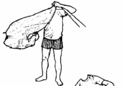
**29)** As it lies on the floor, the bundle should be triangular in shape, as shown. Note: The slider should be wrapped up in the tail and should stay that way as you stuff the canopy into the deployment bag.
