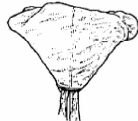
**30)** Dress canopy to a width slightly wider than the bag. All the slider should stay inside the rolled tail. The slider must not be allowed to move down the lines—even the smallest downward movement of the slider may increase opening shock and decrease reliability. Pay extra attention to the position of the slider until the bag is closed.
