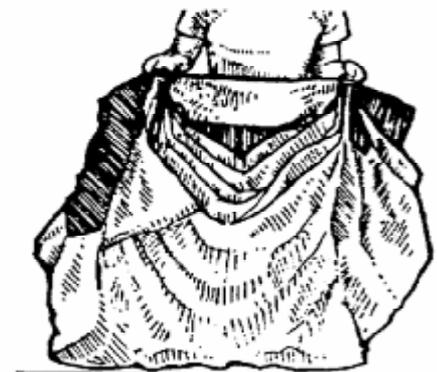
**5)** The nose openings should be facing the rig and the tail should be farthest from the rig. If the reverse is true, double check to be sure the rig is container-side up (the back pad is on the ground). If the rig is positioned correctly and the canopy is not oriented as described above, then the canopy was attached to the harness backwards!
