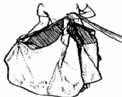
**19)** Fold the D-line group in with one motion to put a real fold in the fabric between the C and D lines. Do the same thing on the other side.
