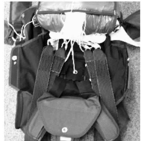
**# 7** ..underside of the bag around both ends of the pull-up cord that was passed through the locking loop. Carefully pull on the other end to pull the locking loop through the packed canopy. Untie the other pull-up cord and set it aside. Place the bagged canopy in the pack tray—taking extra care to fill the lower corners. Then use the pull-up cord to pull the .....
