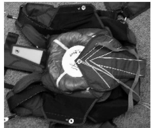
**# 15** Close the right top flap #4 and secure it with the TLP you used on bottom flap #3.
