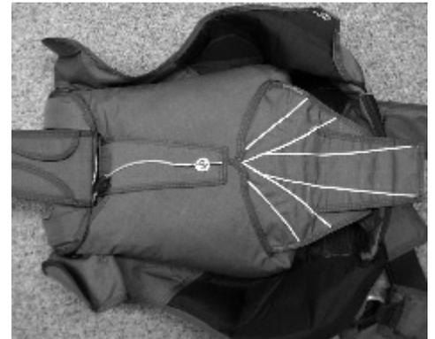
**# 18** Insert the ripcord handle into its pouch on the main lift web.
