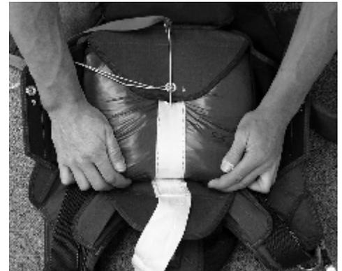
**# 10** S-fold one third of the bridle (5-6 small folds) on top of the free-bag (underneath top flap #2) .
