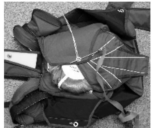
**# 16** Close the left top flap #5 and secure it with the TLP you used on top flap #4.
