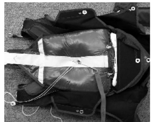
**# 8** ..locking loop through the bagged canopy. Secure it with a temporary locking pin. Now thread the pull-up cord through the grommet on the lower #1 bottom kicker-flap. Pull the locking loop through and secure it with the temporary locking pin – the same one you used before! Bottom kicker-flap #1 also contains the Cypres cutter.
