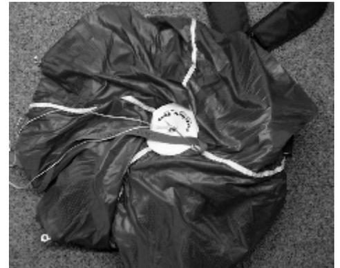
**# 14** Lay the fabric flat all around the P/C and fold it under in wide folds to the center. Fold the top and bottom first, then the sides. Keep the fabric folds out from under the open flaps. Now close the bottom #3 flap and secure it with the TLP you used before.
