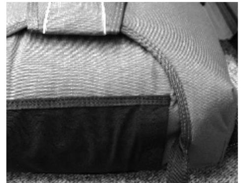
**# 9** Make sure that your main risers are exactly placed on top of the lower closing flap of the reserve container.
