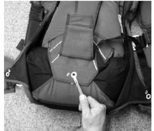
**# 5** Now thread the pull-up cord through the grommet on the #3 flap on the right...
