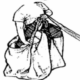
**20)** Now grasp the steering lines where they attach to the tail, pull the entire tail out and drop it straight down.
