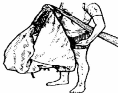
**13)** Clear the stabilizers. Since all lines are bunched up in the middle, pull each stabilizer panel out one by one into a loop until they form an irregular shape resembling the petals of a flower when viewed from the top. Be sure none of the lines are wrapped around a slider stop on a stabilizer.
