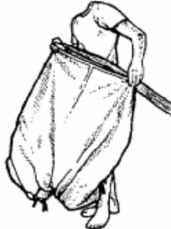
**25 & 26)** Release your knee grip on the nose and tail. Take both tail pieces in one hand and roll them together into the middle so they completely encase the rest of the canopy.
