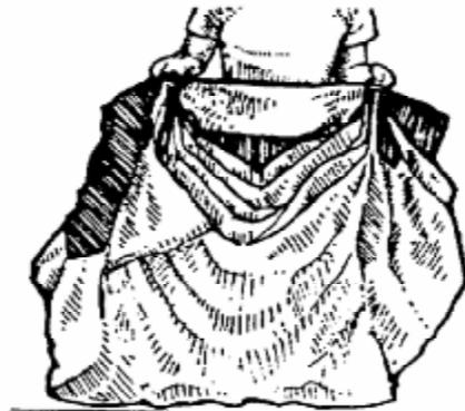
**5)** The nose openings should be facing the rig and the tail should be farthest from the rig. If the reverse is true, double check to be sure the rig is container-side up (the back pad is on the ground). If the rig is positioned correctly and the canopy is not oriented as described above, then the canopy was attached to the harness backwards!
