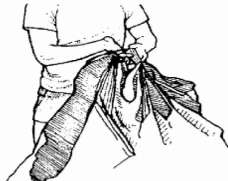
**6)** Now step to one side outside the lines and transfer the lines to one hand so that the left and right sides of the canopy hang at the same height. It is not necessary to keep the line groups separated by the fingers of your hands because you've already determined the lines and canopy are straight. Your canopy should look like the illustration. All lines should be kept taut and the nose should still be facing the rig. The slider should be against the slider stops on the stabilizers.
