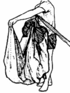
**23)** On one side, start with the middle of the tail being held under your thumb and pull the excess material straight out. You're pulling out the trailing edge of the canopy that extends from the inside steering line to the very center of the trailing edge.
