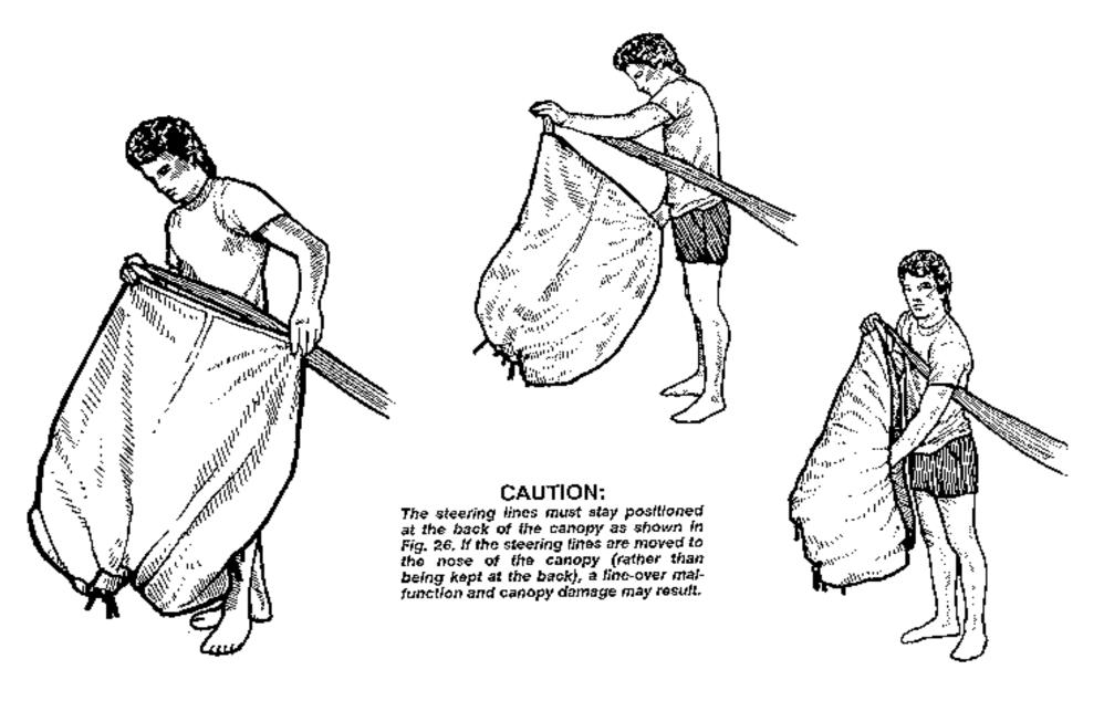
28) Reach down and pick up the very middle point of the trailing edge; an identification marker is sewn at the middle point to help you. Raise the tail a couple inches above the slider and hold it in place with the same hand that is holding the lines.
