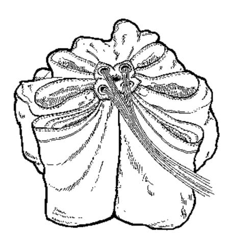
in front of you as you have it now, the A lines are the front part of the line group that go through the front slider grommets, the ones that should be closest to you.
