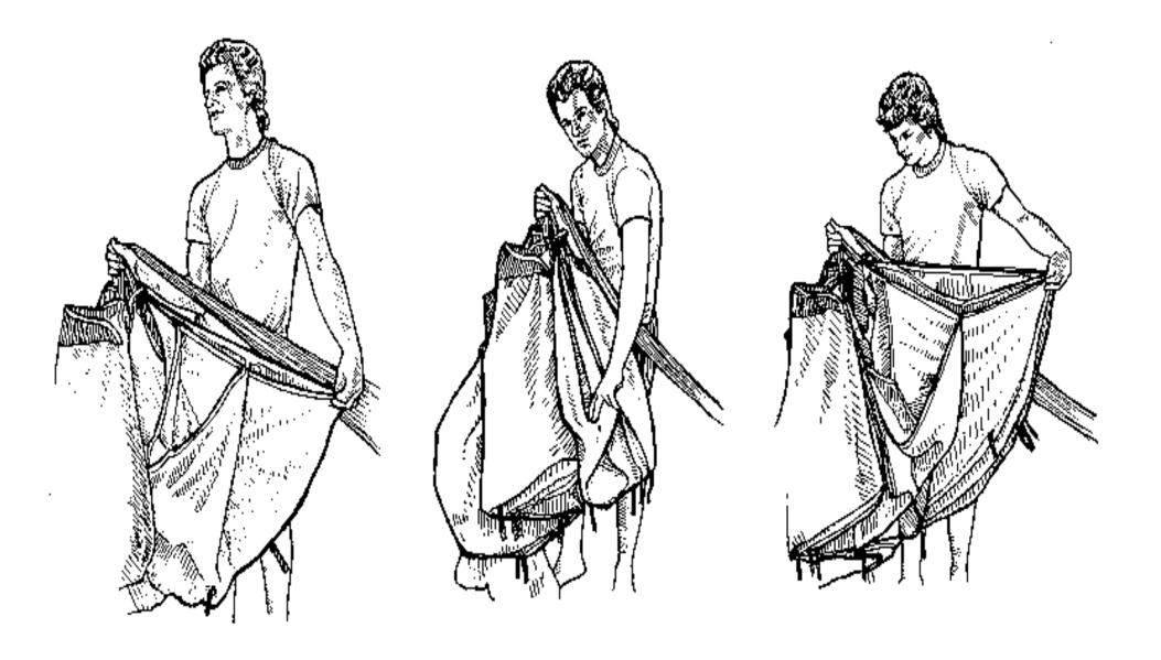
7) Starting with the end cell nearest your legs, flake the entire nose with one hand as shown.
