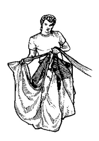
25) Now grasp the steering lines where they attach to the tail, pull the entire tail out and drop it straight down.
