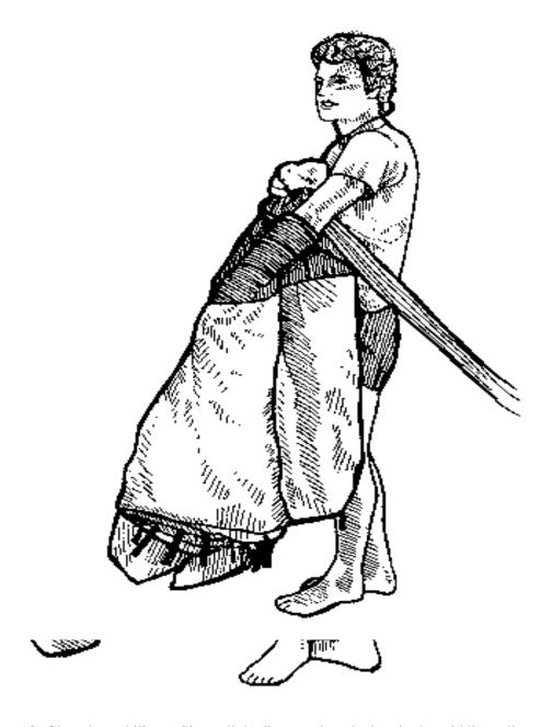
18) Clear the stabilizers. Since all the lines are bunched up in the middle, pull each stabilizer panel out one by one until they form an irregular shape resembling the petals of a flower when viewed from the top. Be sure none of the liens are wrapped around a slider stop on a stabilizer.
