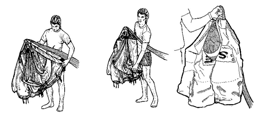
12 & 13) Loosen your knee grip on the nose of the canopy. Find the very middle of it (by running your hand down between the front two slider grommets; exactly half the lines will be on one side and half on the other). While leaving the very middle cell hanging, pick up all the others on one side and roll them in towards the middle.
