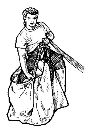
24) Fold the D-line group in with one motion to put a real fold in the fabric between the C and D lines. Do the same thing on the other side.
