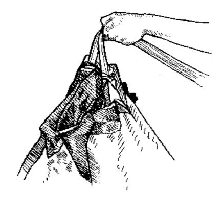
5) The nose openings should be facing the rig and the tail should be farthest from the rig. If the reverse is true, double check to be sure the rig is container-side up (the back pad is on the ground). If the rig is positioned correctly and the canopy is not oriented as described above, then the canopy was attached to the harness backwards!
