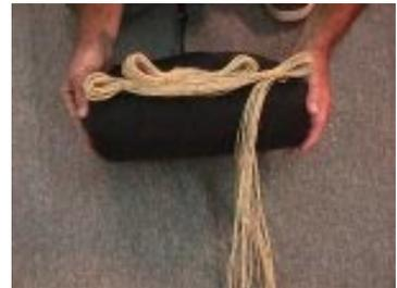
Close the bag and stow lines according to container manufacturer's instructions. It is important to use proper stows (Use stow band material specified by the container manufacturer). We recommend making a double turn with all stow bands, to help prevent line dump.
