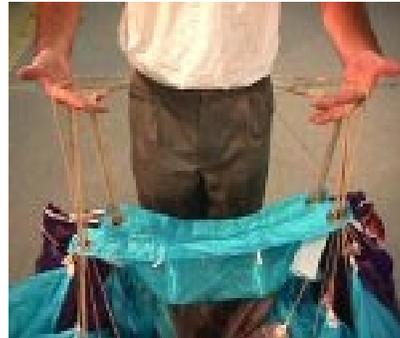
Determine that the suspension lines are straight by separating the four line groups as well as the control lines and clear the lines up to the canopy.
