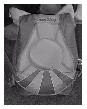
This procedure assures that every TEAR DROP 1 PIN has the right loop length for a good pack job and an easy ripcord pull. The CYPRES loop does not stretch and allows the ripcord to slide more easily than a nylon loop would, even when the reserve pilot chute is pulled firmly down on the container.
