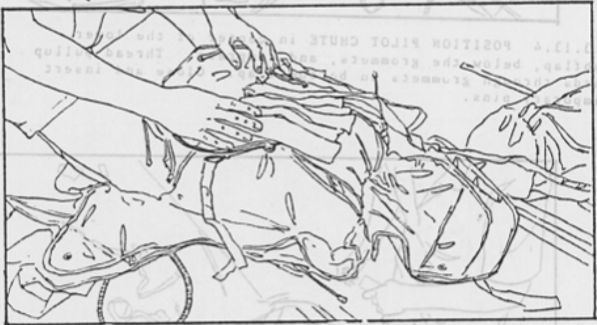
3.3.13.3 S FOLD BRIDLE line on top of the subflaps in seven-inch folds. Spread it out between side flaps.
